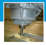
Global aircraft industry (Airbus, Boeing, ...), which is naturally very demanding in terms of machining process quality, is gradually equipping its machining centres with miniaturized and optimised micro-lubrication systems.
